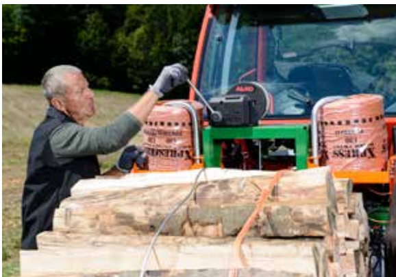
The bundle of wood is pre-tensioned with the aid of the winch.
