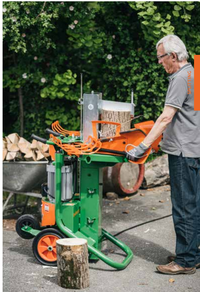
SpaltAxt 10 comes with a 26-cm splitting knife that allows for the processing of even greater wood diameters (up to 40 cm).
