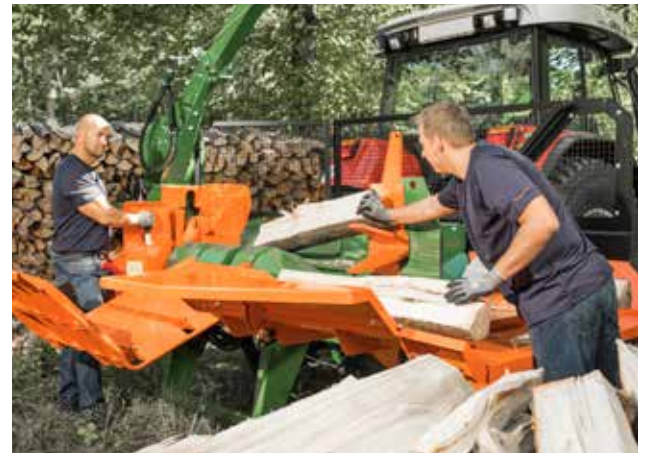
With the standard safety package, several people are allowed to work on the SplitMaster.
